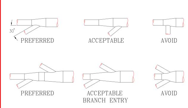
Branches should enter at gradual expansions and at an angle of 30° or less (preferred) to 45° if necessary. Expansion should be 15° maximum. See Fig. 5—15 for loss coefficients.
