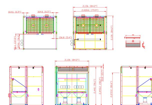
WB-7078G w/SDT-81 GRINDING BOOTH w/Downdraft table SPECIFICATIONS
