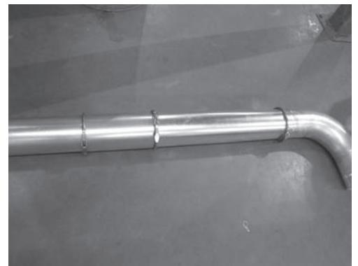
For lengths under 11", mark the duct approximately 2" shorter than the needed length.
