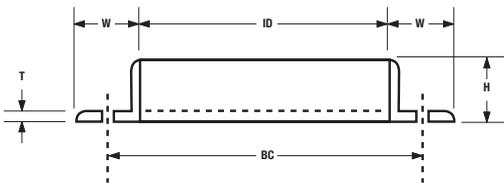
**Note:** Gaskets are in stock for Kirk & Blum rings in sizes 3" through 50". They are 1/8" thick black neoprene and punched to K&B specifications. Other gasket materials are available as a special order.
