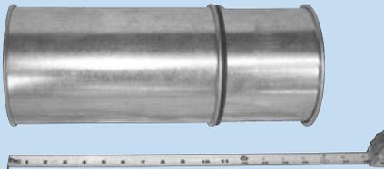
The sleeve is 11" long and therefore the shortest length of adjustment is 11". Additional 'adjustability' for lengths shorter than 11" is provided for in the collars on all fittings. To utilize, simply cut a standard piece of duct slightly longer than the needed length. Place an O-ring over the cut end and slide into the fitting. Once the desired length is obtained, clamp the O-ring to the rolled lip on the fitting. ORDER EXTRA O-RING.
